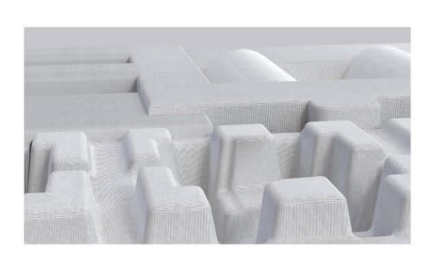
The pulp part is formed to shape by custom designed tools. The tools are lowered into the pulp mixture and the water is pulled through the mesh with a vacuum. The upper tools press into the lower tools to help shape the pieces. Suction from the vacuum helps bind the fibers. After forming, the parts are wet and need to be dried.
