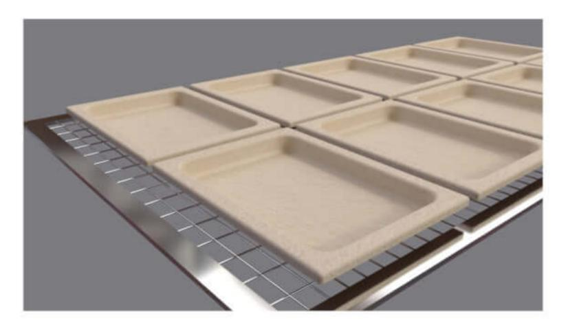
Traditional molded pulp packaging (dry press) is dried on open air drying racks. Thin-walled (wet press) molded pulp packaging is dried with automatic, high temperature and pressure drying machines.
